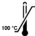
The bottles and jars used must be resistant up to temperatures of **at least 100 °C**. The device is therefore not suitable for polyethylene (PE) bottles or breast milk bags.
